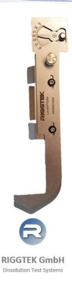
The RIGGTEK "Level Probe" is a special gauge for accurately set the paddle or basket height in all high-head Dissolution Testers or for validating the height of each stirring element precisely in seconds.
